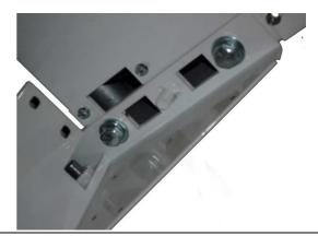
3. Retrieve the motor cords (black outer wrap) and microwave sensor cords (grey outer wrap) from the rectangle openings. Then, connect the cords with the extension cords from the rectangle openings on the top end of the pillars. Place the cords behind in the cord-trough inside the right pillar.
