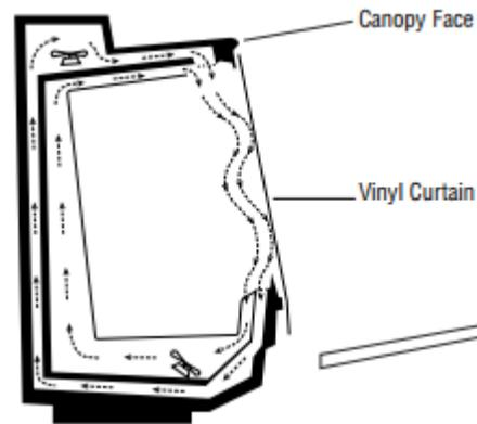
Simply Peel back the Velcro to access the cooler for product stocking or cleaning...
